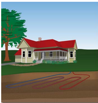
Horizontal ground loop
