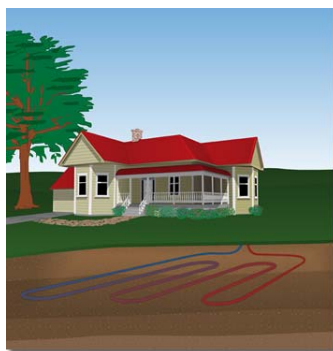
Horizontal ground loop
